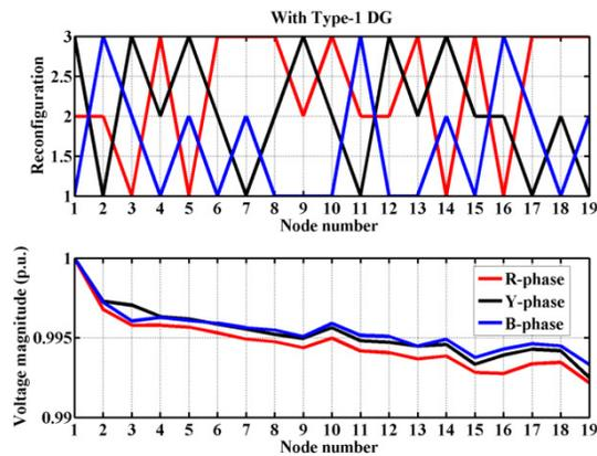
**Fig. 9.** Variation of node voltage and phase reconfigurations with Type-1 DG for URDS-19 node system.
