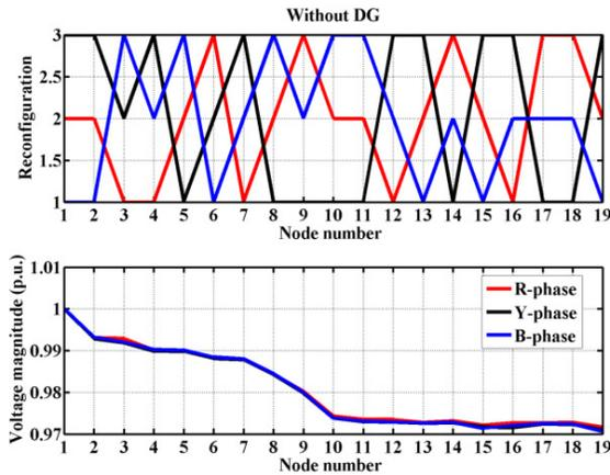
**Fig. 8.** Variation of node voltage and phase reconfigurations for without DG for URDS-19 node system.
